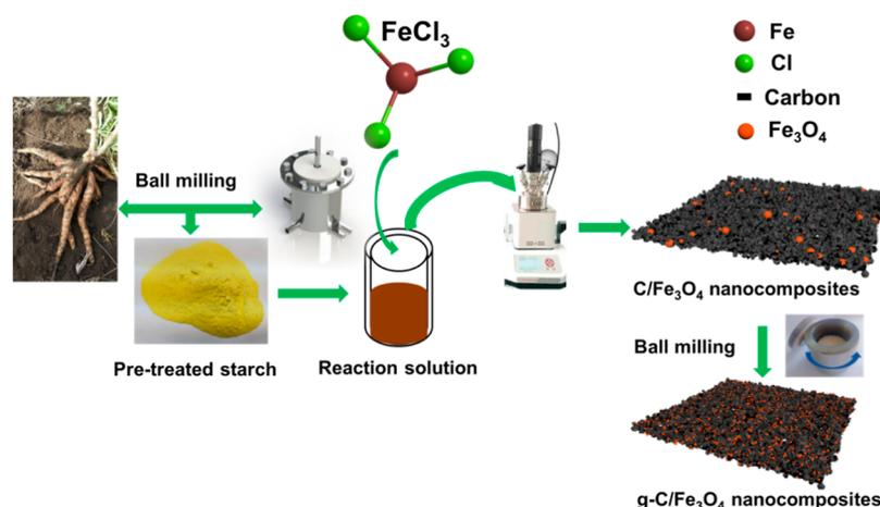
Figure 1. Synthesis schematic of the g-C/Fe<sub>3</sub>O<sub>4</sub> nanocomposites.
